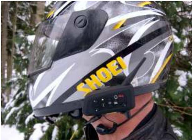
Now it is easy to hook the bluetooth unit into the mounting plate on the helmet outside.
