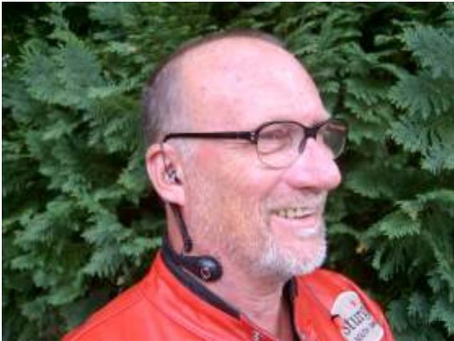
Place the Neck-band around your neck, see to so that the microphones pick-up plate is in good contact with your skin. You may bend the Neck-band to ensure the proper connection to the neck-skin. The best location is to have the pick-up around 4-5 cm beside the voice-box.
